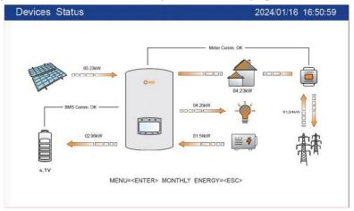
The screen will be automatically turn off after being idle for a few minutes to save power, click any operation button ("ESC"/"UP"/"DOWN"/ "ENTER") to restart the screen, then press "Enter" into the main operation interface.
