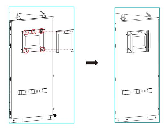
3. Lift up the PCS, and align the back bracket on the PCS with the convex section of the mounting bracket. Hang the PCS on the mounting bracket and tighten the screws on both sides to secure the PCS.
