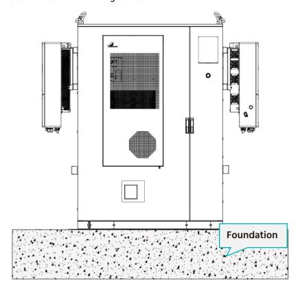
• The cabinet is fixed at the bottom, and holes should be pre-opened on the installation site in accordance with the positioning holes at the bottom of the cabinet. See the drawing below.
