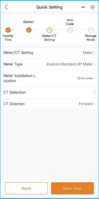
Method 2: Setting --- Professional Setting -- Device Setting -- Meter/CT Setting
