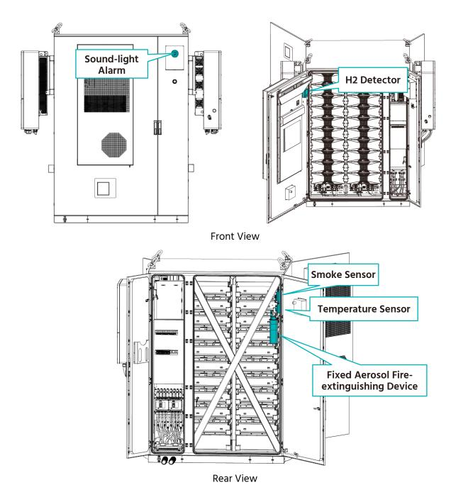
The outdoor battery cabinet is equipped with an aerosol fire extinguishing solution. And the cabinet is equipped with a fire extinguishing device. The fire extinguishing mechanism of aerosol is mainly reflected in two aspects:
