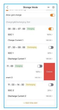
Charge SOC: battery charging stops when reach the set SOC;
