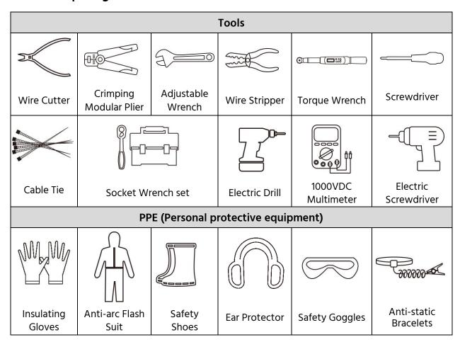
**NOTE:** Use properly insulated tools to prevent accidental electric shock or short circuits. If insulated tools are not available, cover the entire exposed metal surfaces with available insulated alternatives, except their tips, with electrical tape.
